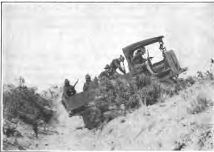
CLIMBING IN AND OUT OF A GULLEY LIKE THIS LOOKS VERY HARD. THE FRONT WHEELS PULL WHILE THE REAR WHEELS PUSH
